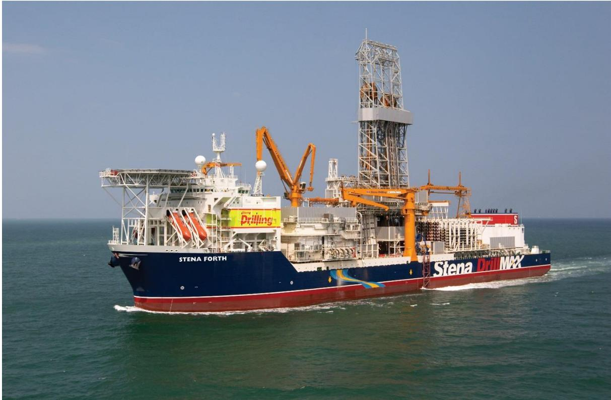
Stena Drilling "Stena FORTH" Dynamically Positioned Drillship
